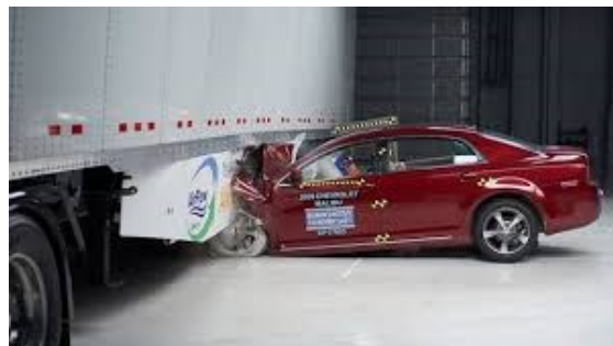
Above: IIHS crash test into tractor-trailer equipped with an Angel-Wing side impact guard on August 29, 2017, at the Second Underride Roundtable. 40 mph
