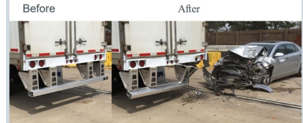
Modified version of the IIHS TOUGHGUARD 30% Overlap Semi-Trailer Underride Evaluation Crash Test Protocol
