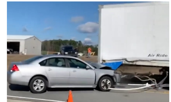
Modified version of the IIHS TOUGHGUARD 30% Overlap Semi-Trailer Underride Evaluation Crash Test Protocol
