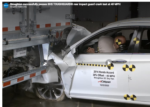
Stoughton RIG Crash Test 40 mph 12/2025
