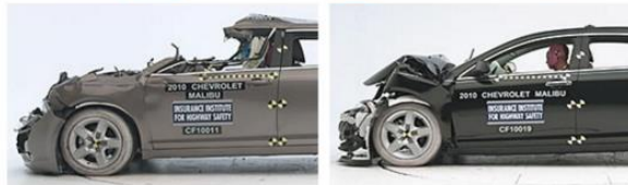
This is how a car looks after a 35 mph full-width crash into the rear of a Hyundai trailer with a weak underride guard.
