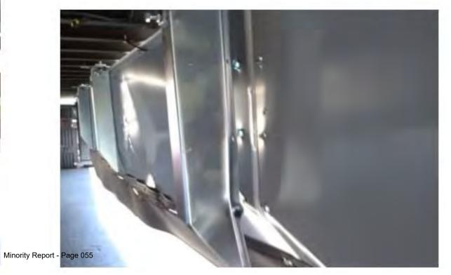
Angelwing Rigid Side Impact Guard Reduces Trailer Ground Clearance Resulting In High Centering Damage To Itself And The Trailer's Structural Integrity
