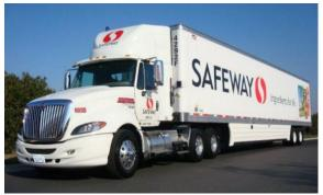
Figure 9: Photo of a Combination Truck (CT) with Aero Side Guard
