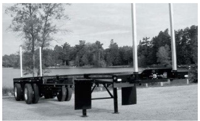
Figure 37: Truck trailer with bolsters (vertical posts). (Source: FMCSA)
