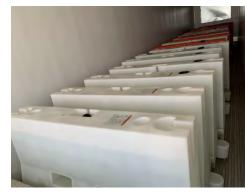
40,000 Pound Payload in Trailer (vs 22,487 at IIHS) (Utility *trailer moved approx. 3" at impact.*)
