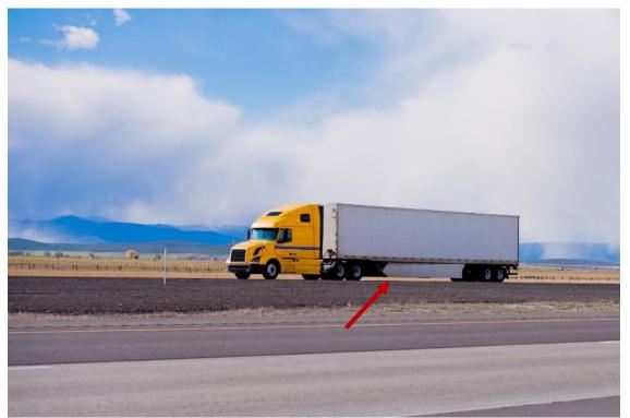
Figure 45: Truck with aerodynamic skirt. (Source: Vitpho, 123rf.com)
