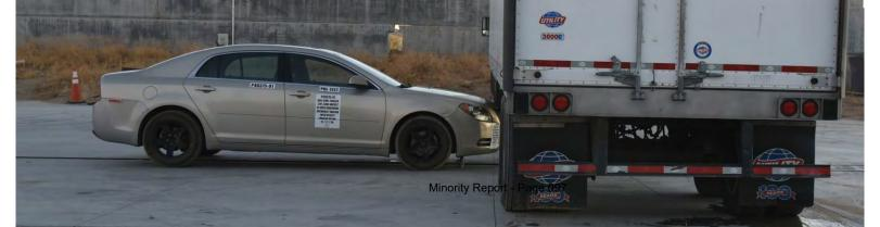
40,000 Pound Payload in Trailer (vs 22,487 at IIHS) (*Trailer moved approx.* 3" *at impact.*)
