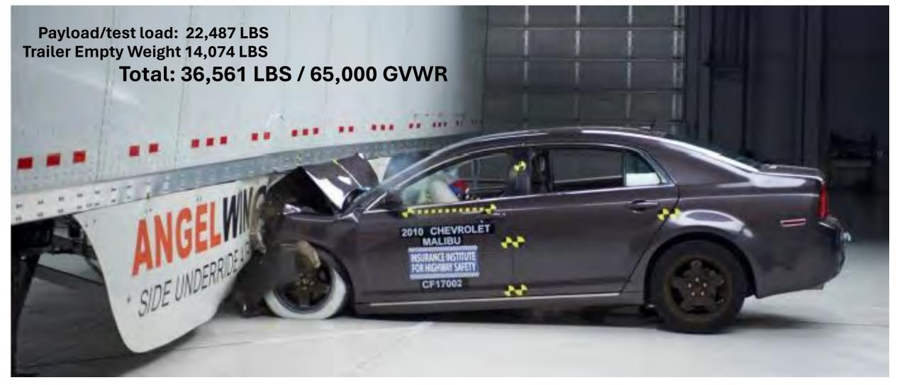
2<sup>nd</sup> Test of AngelWing Side Guard Aug-2017 40 mph / 90-degree impact Payload/test load: 22,487 LBS • Trailer Empty Weight 14,074 LBS Impact Point – center of guard (no other • Total: 36,561 LBS location or angle tested) 2009 CHEVROLE
