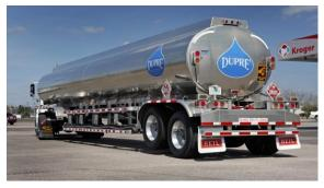
Figure 7: Photo of a Combination Truck (CT) with Rail Side Guard
