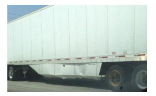
Earlier Aerodynamic Trailer Side Skirt Designs Were Too Rigid To Avoid Ground Damage
