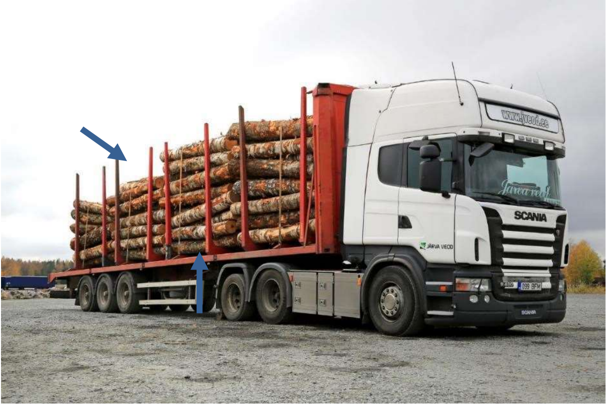
Figure 38: Truck trailer with bunks (horizontal structure) and stakes (vertical structures). (Source: Taina Sohlman, 123rf.com)
