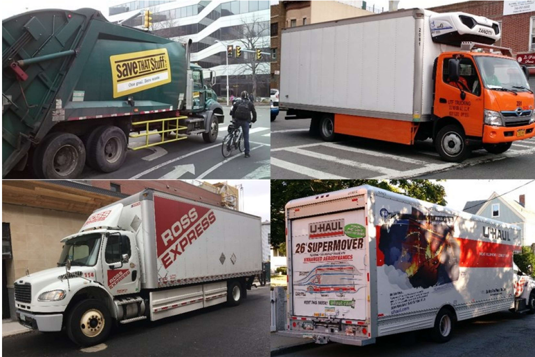
Figure 33: Private sector rail and panel style side guards in the Boston and New York City (NYC) metro areas (Source: Volpe)
