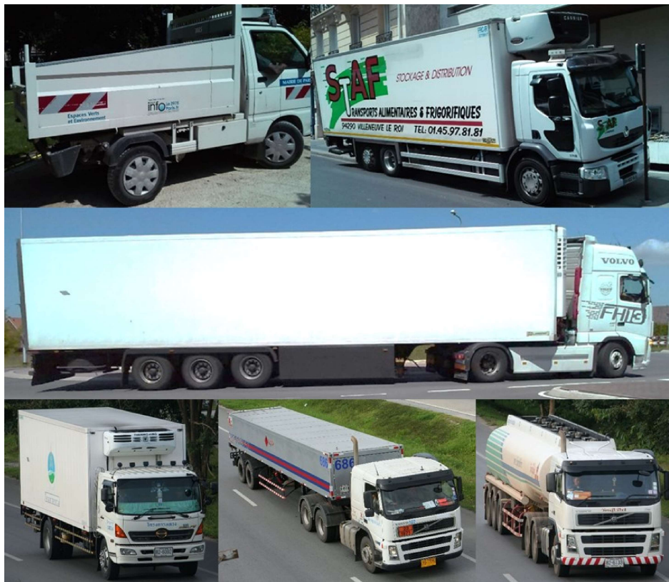
Figure 3: Images of UN Regulation 73 side guards in France (top), the Netherlands (middle), and Thailand (bottom) (Source: top and middle, Volpe; bottom, Nuttapong Wannavijid, 123rf.com)
