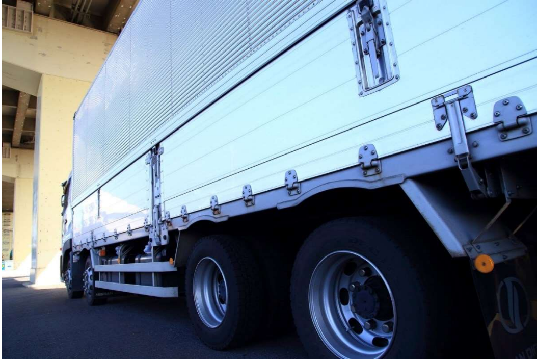
Figure 23: Image showing a rail-style side guard on a truck in Japan (Source: Hirohito Takada, 123rf.com)
