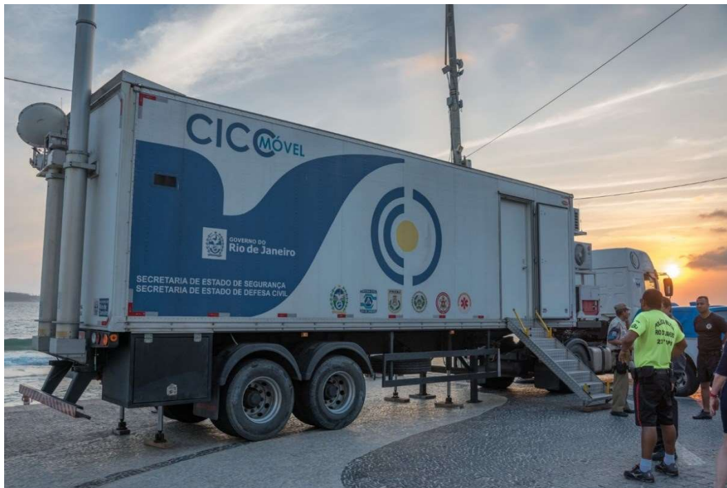
Figure 28: Image showing a side guard on a truck in Brazil (Source: Sergio Shumoff, 123rf.com)
