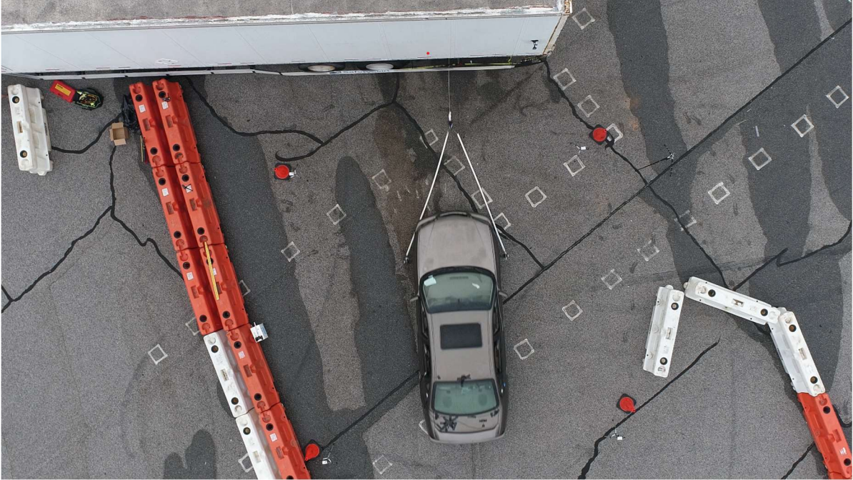
90 Degree Angle Behind Axles Test, Chevrolet Malibu, 35 mph, SafetySkirt Side Guard, 8/2023
