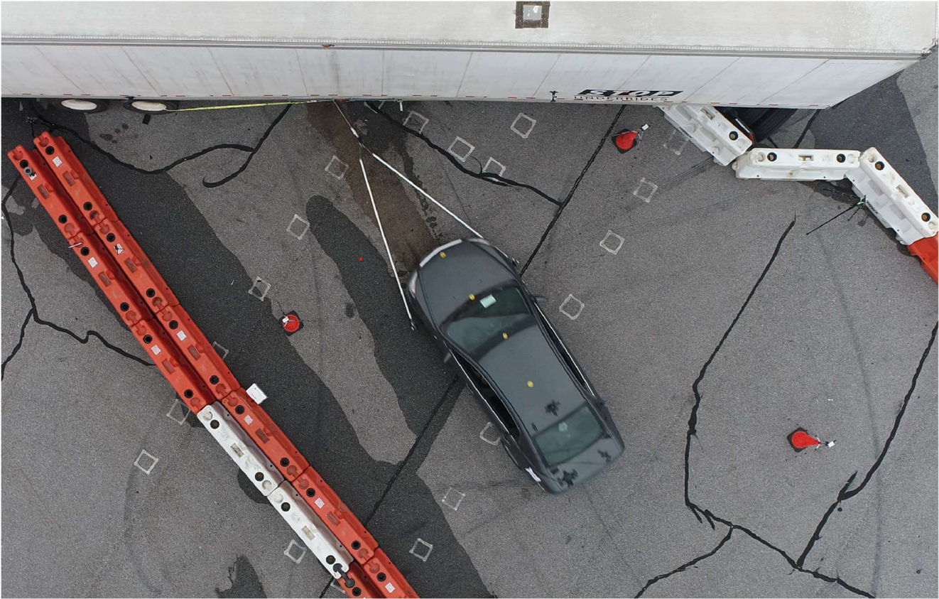
45 Degree Angle Test, Chevrolet Malibu, 37 mph, Unguarded , 8/2023
