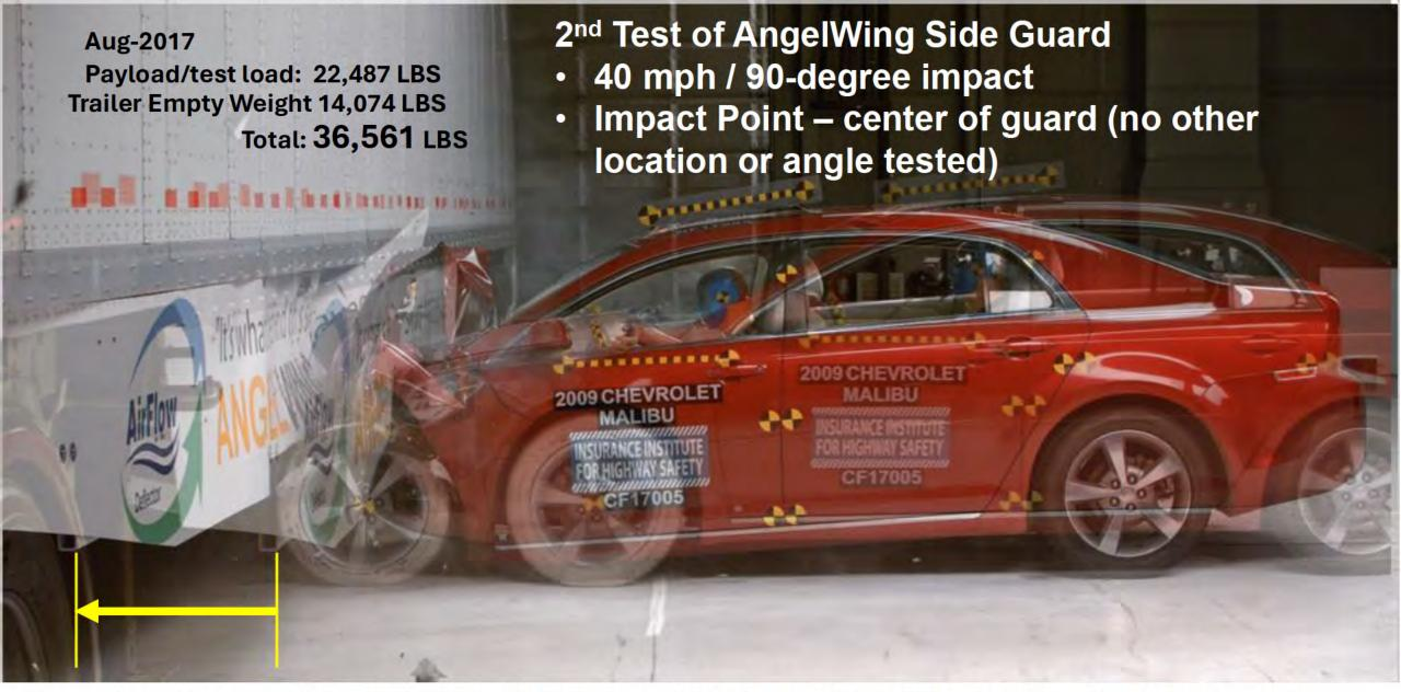
Excessive slide (approximately 24") from impact of trailer (poor test boundary condition – lightly loaded trailer, smooth floor).
