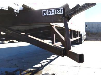
UTM Side Impact Guard was not effective when impacted at one end. This is the only test we know of conducted at 30% (car to guard) overlap.
