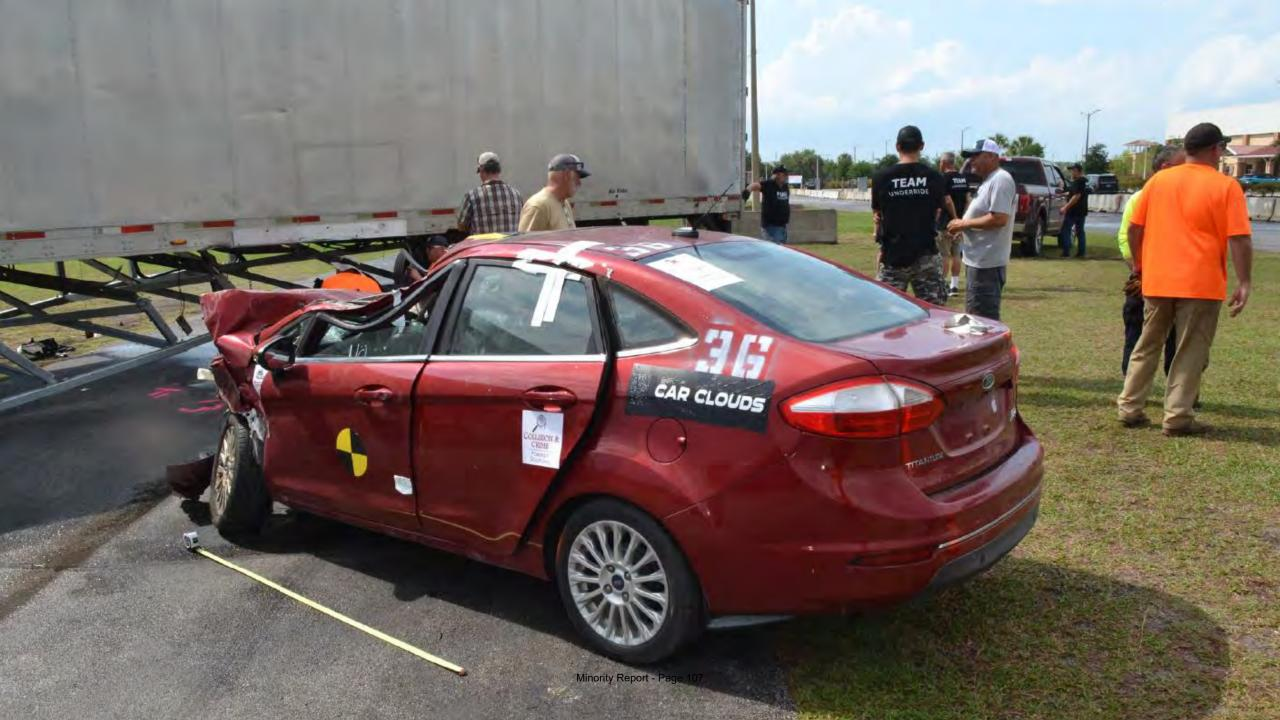
Ford Fiesta AngelWing Test Performed by "Stop Underrides and Collision & Crime Forensic Solutions" Confirmed AngelWing Side Underride Guard not effective in a 45-mph center impact at 45 degrees.
