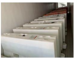
40,000 Pound Payload in Trailer (vs 22,487 at IIHS) (Utility trailer moved approx. 3" at impact.)
