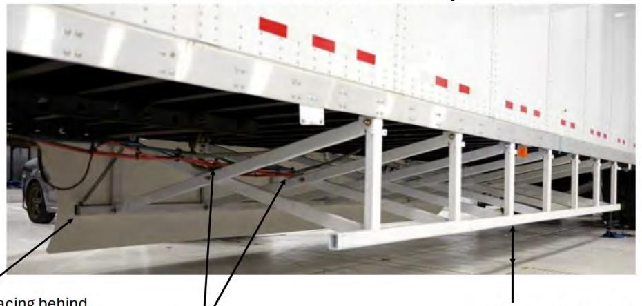
The rigid bracing behind aerodynamic trailer side skirts have instituted DOT safety recalls of specific side-skirt designs.
