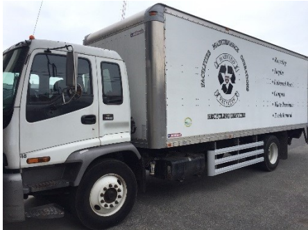
Figure 6: Photo of a Single-Unit Truck (SUT) with Rail Side Guard
