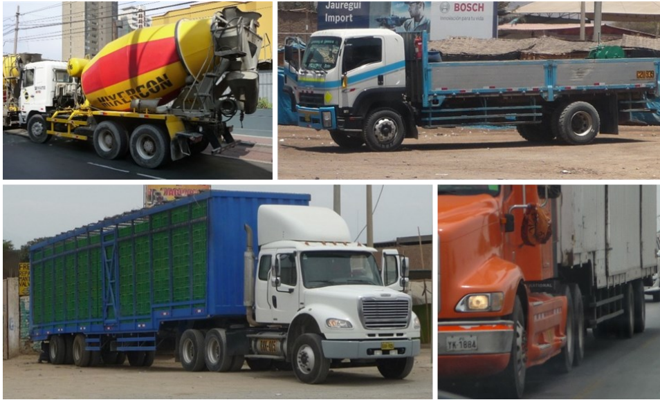
Figure 26: Images of single-unit and combination tractor trailers equipped with side guards in Peru (Source: Volpe)
