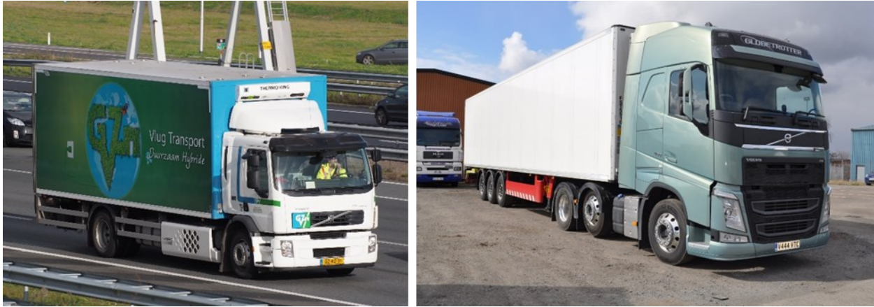
Figure 49: Images of Volvo side guard-equipped vehicles currently manufactured for non-U.S. markets (Source: Alf van Beem and Raymondo166, Wikimedia Commons)
