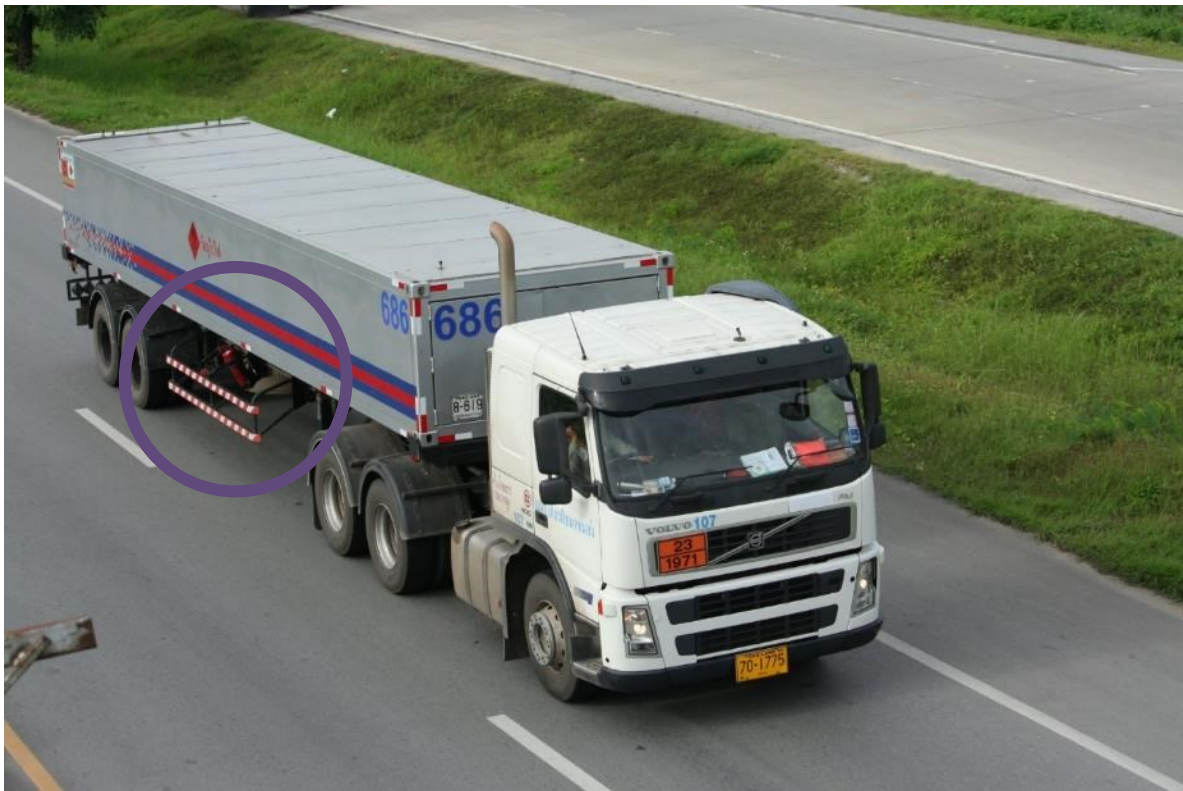
Figure 43: Truck with fire extinguisher behind side guard (Source: Nuttapong Wannavijid, 123rf.com)
