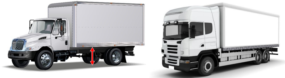
Figure 1: A large truck (left) typically has an exposed space, represented by the vertical arrow and approximately 50 inches in height, between the axles. During a collision, vulnerable road users (VRUs) can fall into the exposed space and suffer fatal crushing injuries. Side guards (right) are designed to cover these exposed spaces. (Source: mechanic, Dan Barbalata/123rf.com)
