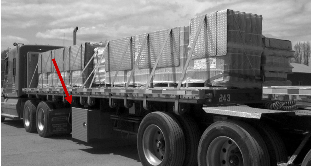
Figure 42: A truck with an underbody toolbox. (Source: FMCSA)
