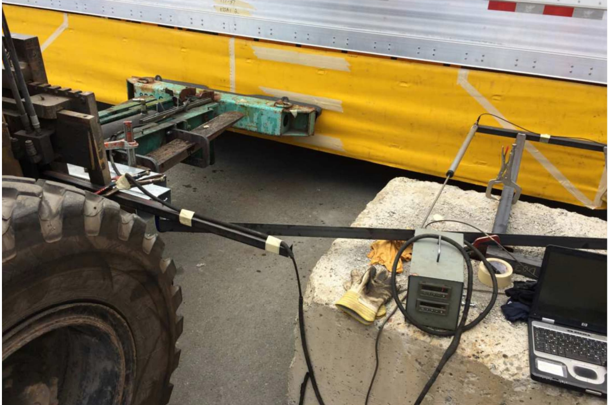
Figure 3: Full Scale testing setup for bumper push test.
