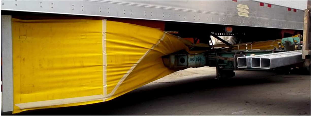
Figure 4: Deformation of SUPD under bumper loading.
