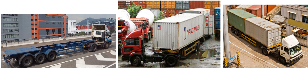
Side guards found on intermodal chassis internationally.
