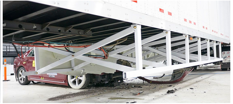
Angelwing Retrofit, 40 mph Test
