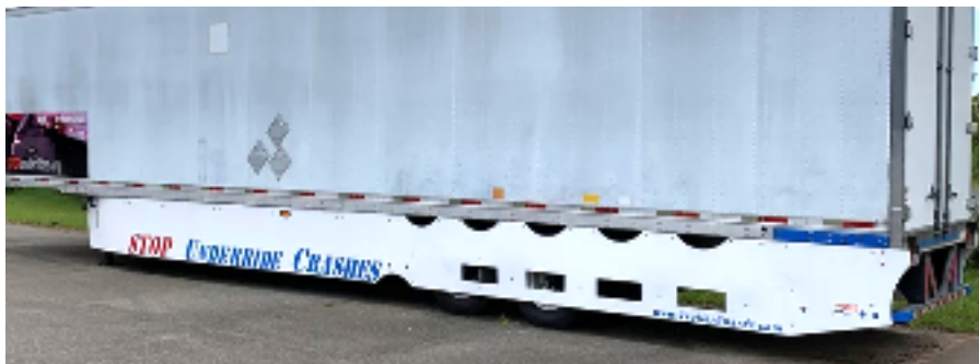
SafetySkirt Retrofit System (Angelwing, SafetySkirt, ToughGuard for max fuel savings and complete underride protection)
