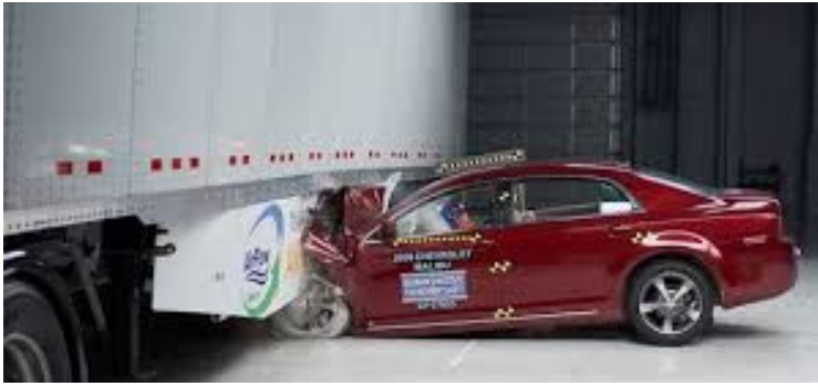
Angelwing Retrofit, 40 mph Test
