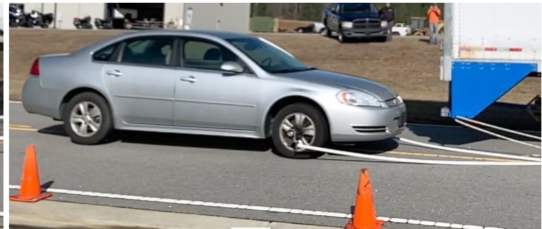
ToughGuard Retrofit, 38 mph / 30% Overlap Test
