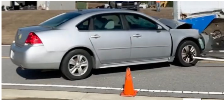
ToughGuard Retrofit, 38 mph / 30% Overlap Test
