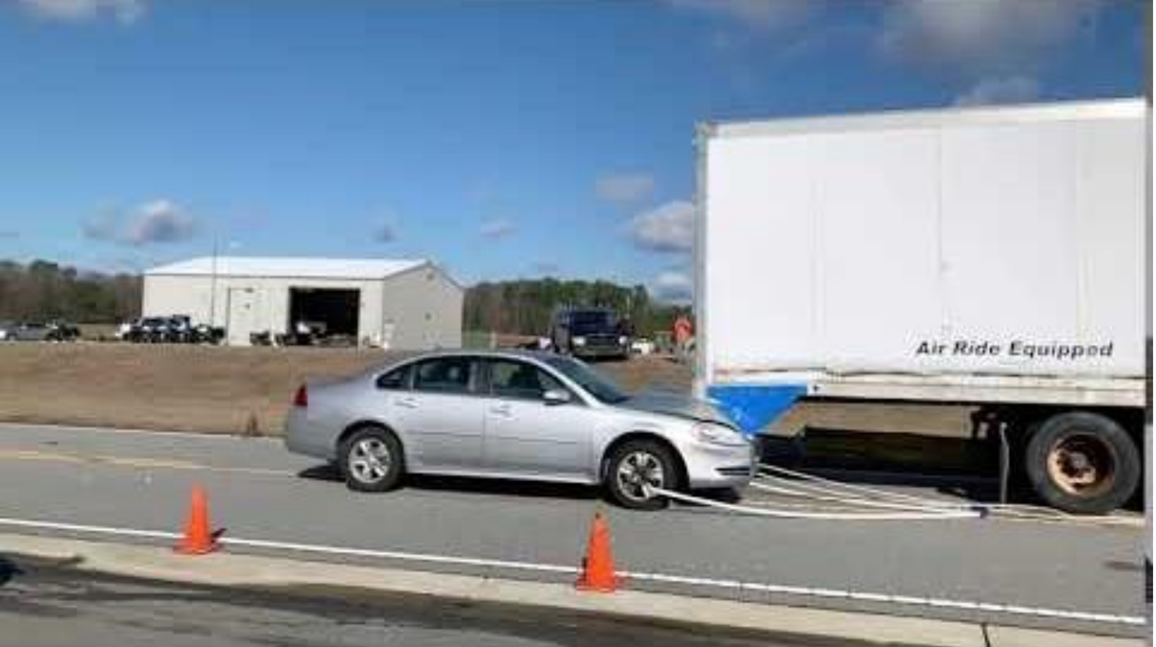
Crash Test of Rear Reinforcement Attachment
