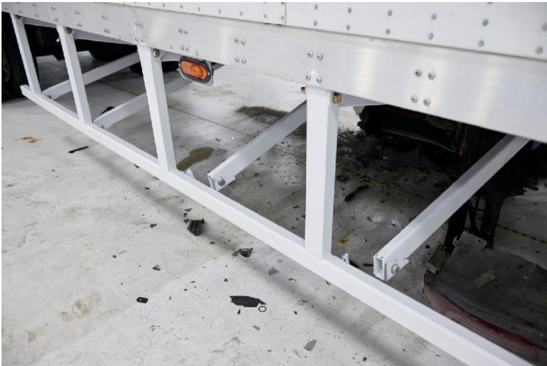
Figure 8 Postcrash – Underride guard damage, nonstruck side of trailer chassis
