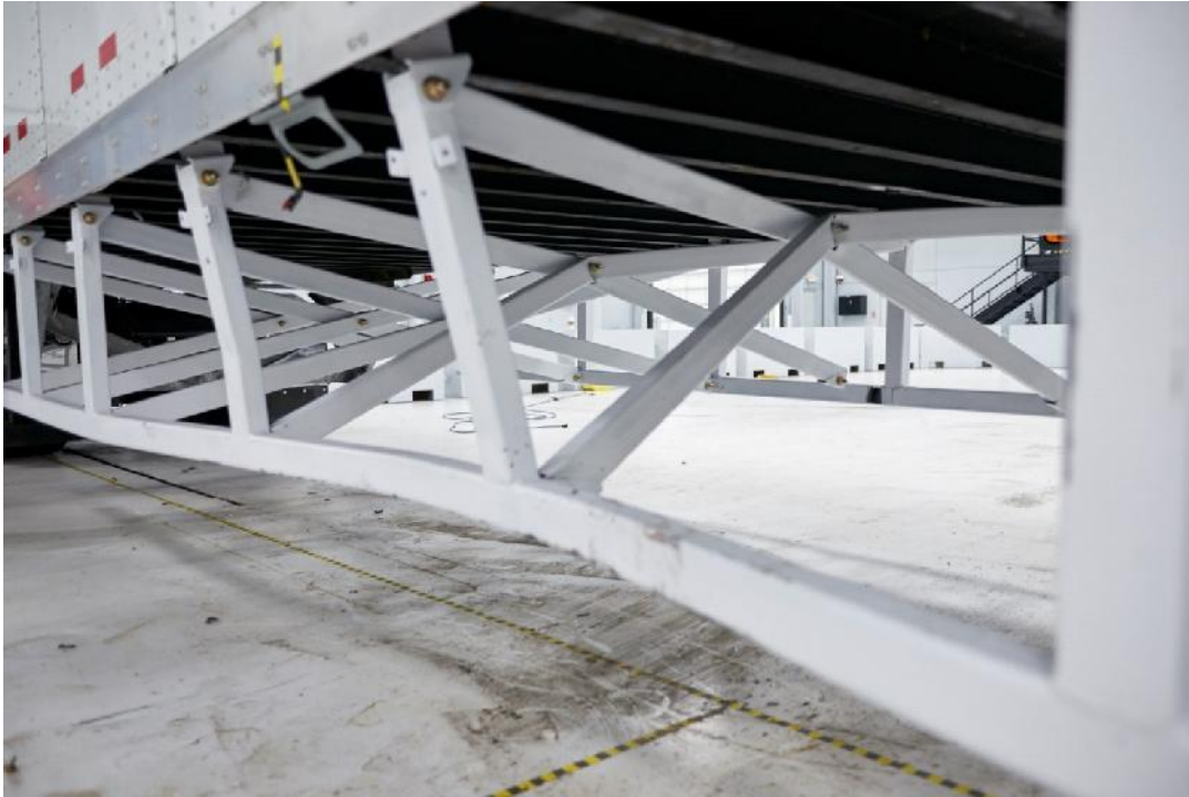
Figure 8 Postcrash – Underride guard damage, nonstruck side of trailer chassis
