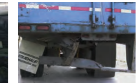
Trailer deck/chassis weakness
