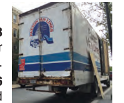
Single-unit truck exempt from NHTSA rear underride guard requirement
