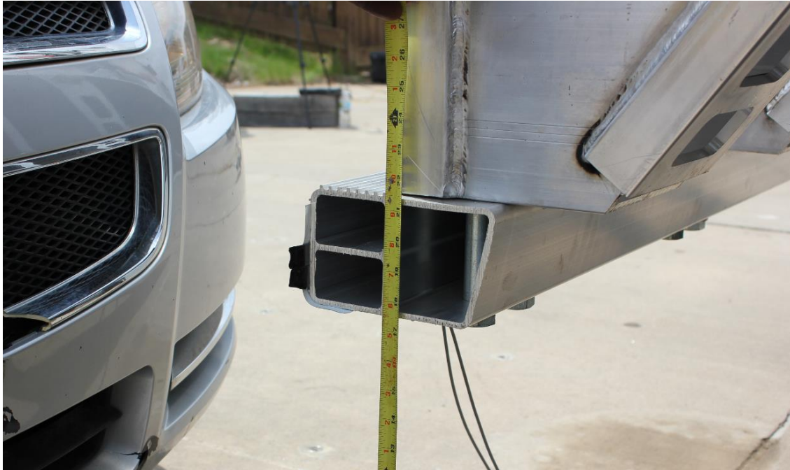
Figure 3 Test Configuration – Bumper Height
