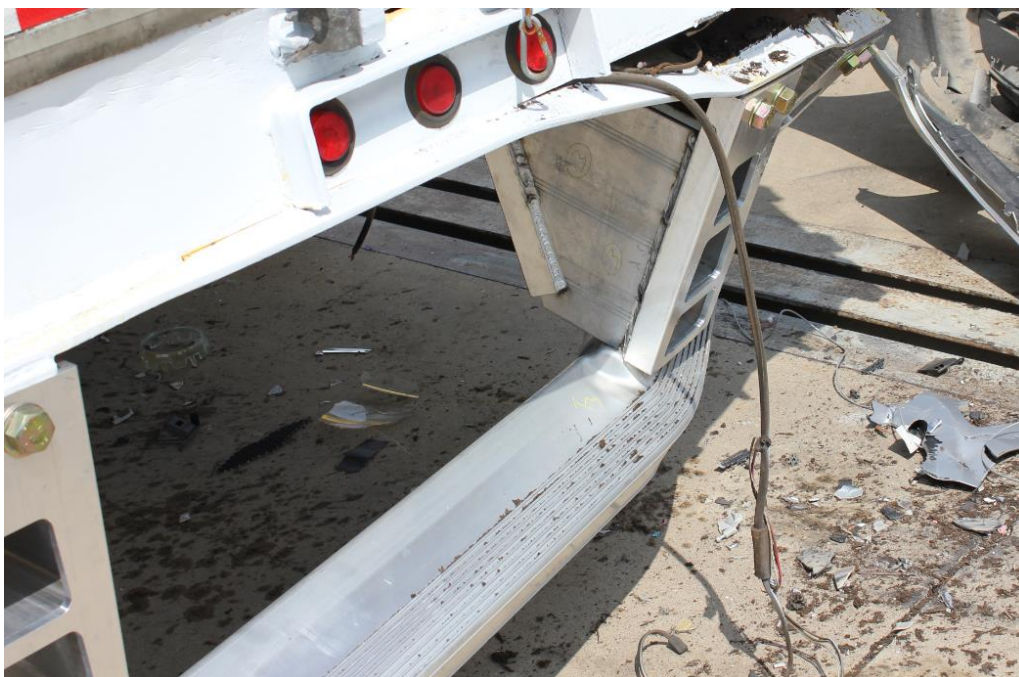
Figure 5 2017 Sapa 40/30 RIG – Post-Crash Right Vertical Support
