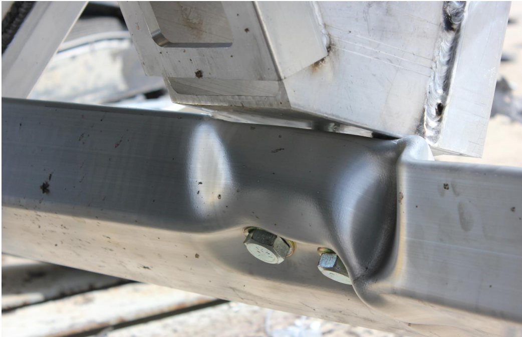
Figure 8 2017 Sapa RIG 40/30 – Post-Crash CA24 Bumper Deformation
