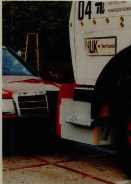
Front-end protection system rides low enough to keep car from sliding under the truck in a crash.
