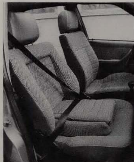
Three-point adult belt together with booster cushion. Seated farther back than an adult, the child will receive better side support and lap belt fit.
