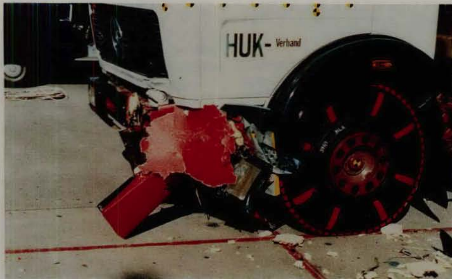
Frontal crash guard absorbs crash force and reduces damage to the truck itself.
