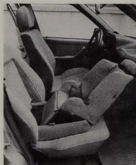
Integrated head rest can be moved up or down. Seat angle can be adjusted.
