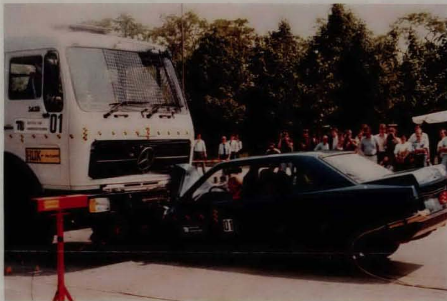
In this test collision, the truck bumper intrudes dangerously close to the passenger cabin.
