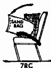
Fig. 34(a) - This seat was additionally loaded by a 100-lb belted sandbag
