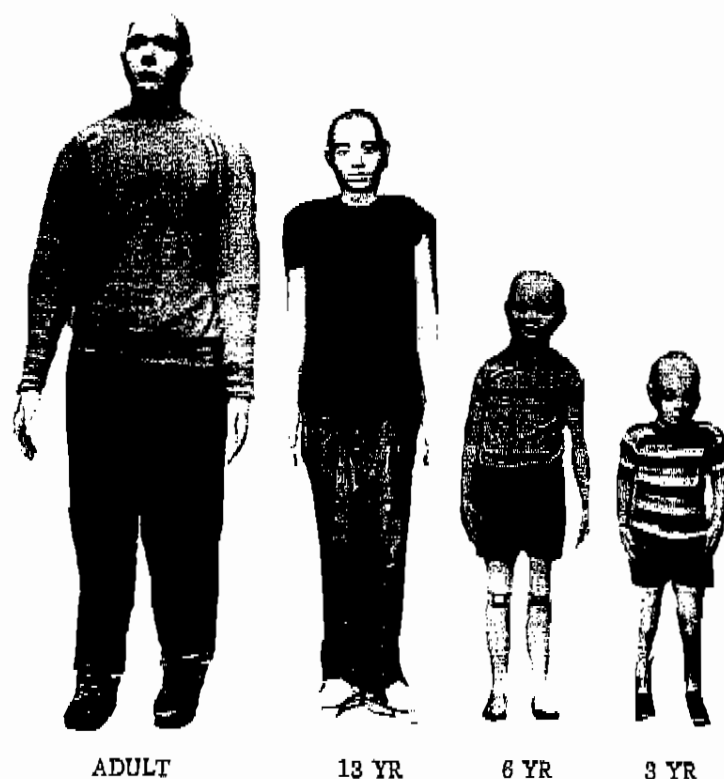
Fig. 6(b) - Anthropometric dummy passengers in UCLA school bus experiments
