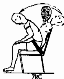
Fig. 52(c) - Lap belt loading (less than 50 lb) occurred on rebound from seat for this rear-end collision
