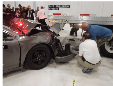
Crash Test with Improved Rear Underride Guard:
