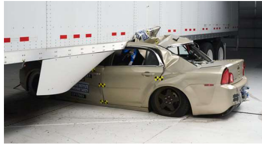
Truck Crash Test Without Side Guard:
