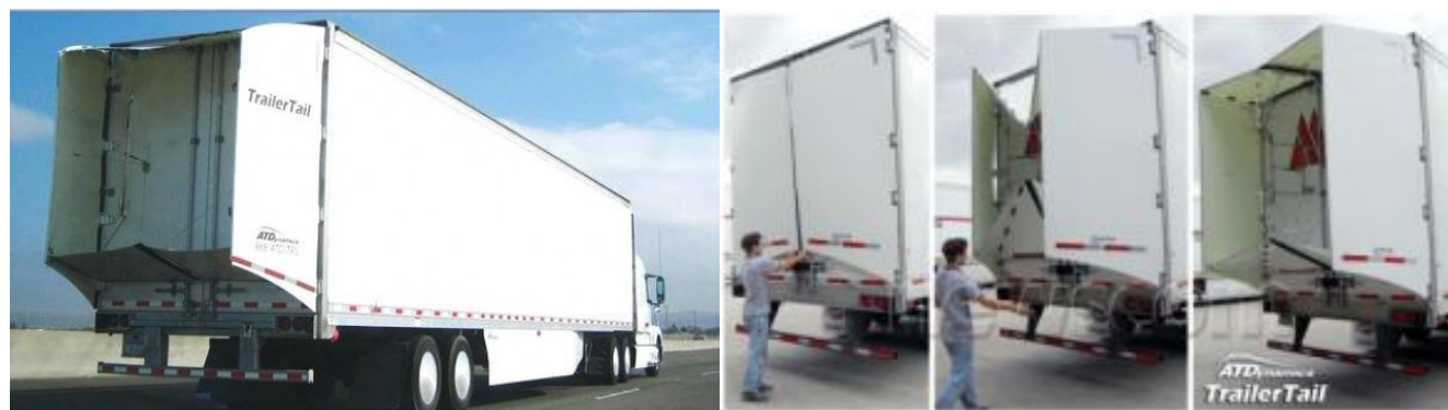
Figure 2: ATDynamics Trailer Tail deployed (left) and stowed (right)
