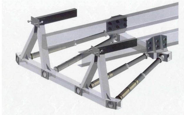
Figure 6.1: MURAC energy-absorbing underride guard
