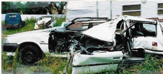
Photo F10-2 Side view of station wagon. A-pillar and B-pillar were torn out by the impact.
