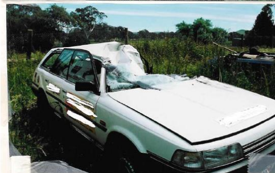
Photo F10-3 Driver's side view of crashed vehicle – note largely intact side structure
