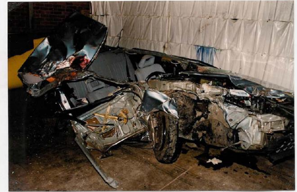
Photo F33-1 Side view of the car, showing flattening of A pillar and shearing of roof back to the C pillar
