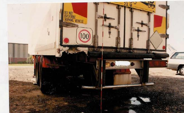
Photo F33-2 Rear view of damaged trailer. Note partial width of underrun bar and damage to the rear corner of the fiberglass body of the van.
