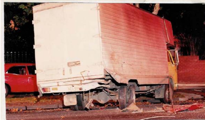
Photo F33-2 Rear view of damaged trailer. Note partial width of underrun bar and damage to the rear corner of the fiberglass body of the van.
