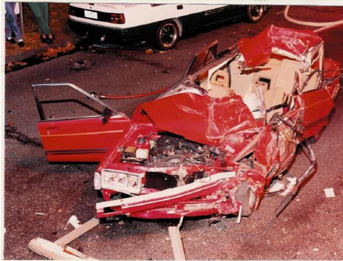
Photo FC12-1 FRONT VIEW OF CAR AT CRASH SCENE. NOTE EXTENT OF ROOF DAMAGE.
