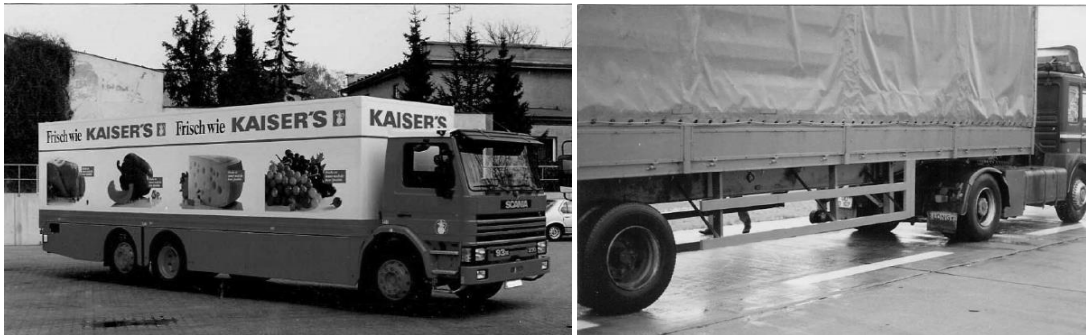
Figure 4: Examples of different side underrun guards on trucks in Europe, comparing flat panels sides (left) with the use of rails (right) (after V. Middelhaue, Germany)
