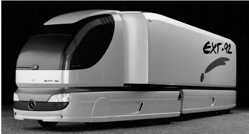
Figure 5: European Experimental Truck EXT-92 shown at the commercial vehicle show Hanover, May 1992. This articulated heavy vehicle illustrates many advanced features including a design which minimises the harm potential to other road users: front and rear underrun protection, smooth side skirts, no projections or sharp edges, spray suppression etc. (Photo courtesy Mercedes Benz Australia)
