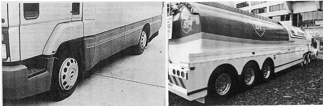
Figure 6: The left picture shows detail of the side skirting of a Ford Truck in Europe illustrating smooth side structure free of protruding edges (V. Middelhaue Berlin Technical University). The right photo is of a BP petrol tanker with side skirts in Melbourne Australia.
