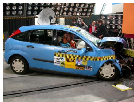
Passenger car after impacting the conventional (left) and the improved (right) underrun protection system.
