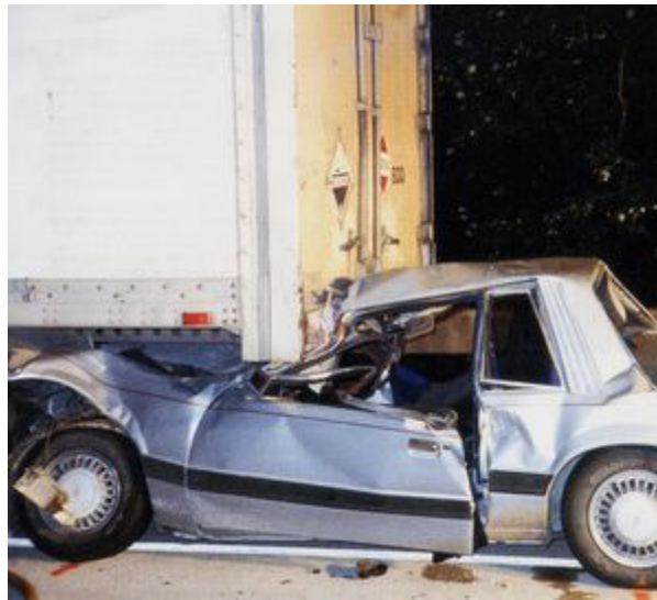
Figure 1. A case of underride from a weak underride guard.
