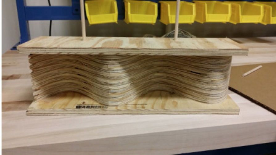
Figure 19. Prototype sine beam built in the Applied Lab using a CNC router.
