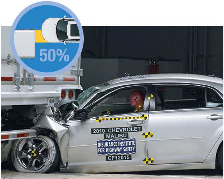
Figure 2. A 50% overlap test using a 2010 Chevrolet Malibu.
