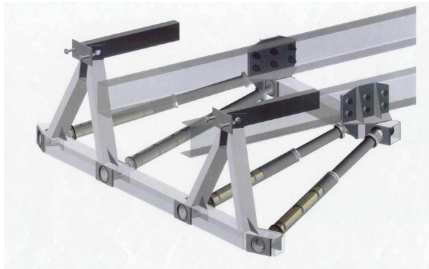
Figure 10.1: MURAC energy-absorbing underride guard
