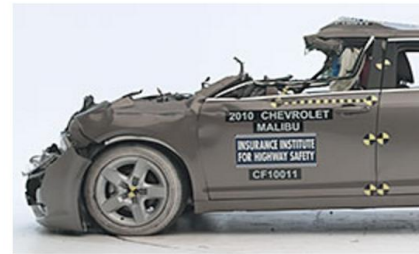
This is how a car looks after a 35 mph full-width crash into the rear of a Hyundai trailer with a weak underride guard.
