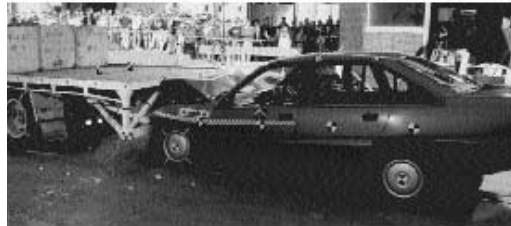
50km/h centre crash, rigid rear underrun barrier, 10t rigid truck
